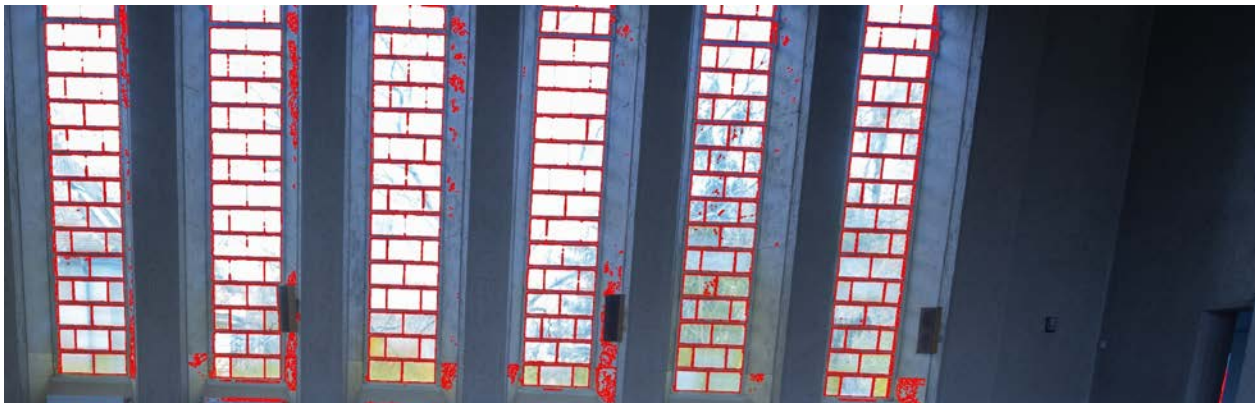
Fig. 2. Example for the automated classification of wooden parts and the texture of a window object as applied on a photogrammetric 3D model of the interior of a church in Leipzig. The errors around the frame can be ignored, as they are outside the borders of the window. The classification system will be applied to every segmented area within an object.
