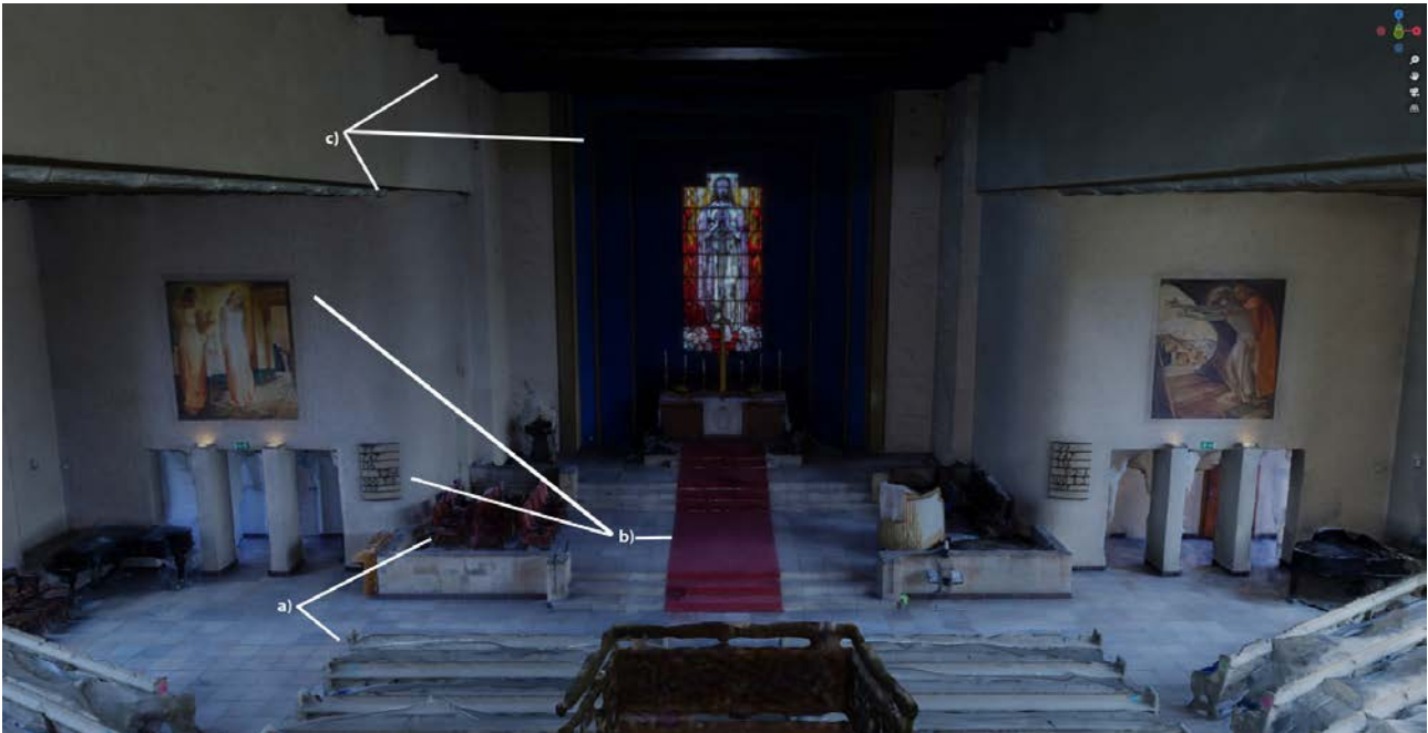
Fig. 1. Photogrammetric 3D model of the interior of a church in Leipzig with different object classifications, a) repetitive objects (chairs & benches); b) different surface structures (painting, plastic and carpet); c) special geometrical features.
